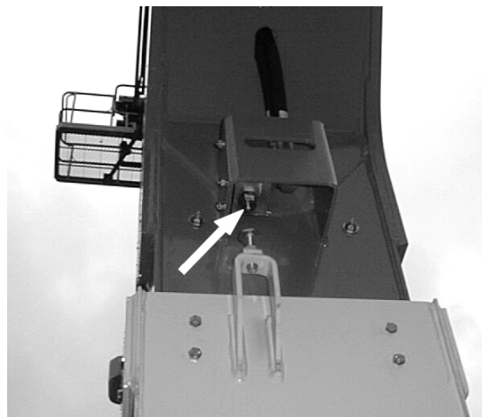
Figure 2-8. Tower Boom Horizontal Limit Switch
